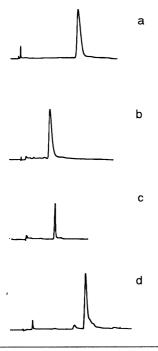
Fig. 1 Reverse phase HPLC pattern of crude homoligomers; Vydac C18 10  $\mu$ m (4.6  $\times$  250 mm), 1.5 ml/min, linear gradient of B solution (50% methanol in 0.1 M TEAA pH 7.0) in A solution (10% methanol in 0.1 M TEAA pH 7.1) during 30 min, a dT<sub>6</sub> (40 – 55% B), b dA<sub>6</sub> (40 – 55% B), c dC<sub>6</sub> (0 – 40% B),
